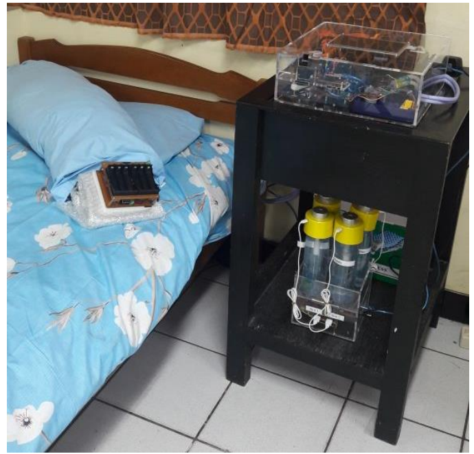
Fig. 9. The smart bed system and warm bolster. The battery module is put inside the bolster as shown in the left side while the other modules are on the black table.
